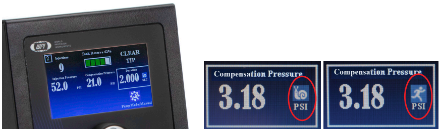
Fig. 17—(Left) Touch the parameter to adjust and rotate the knob to modify the parameter. Fig. 18—(Right) Press the knob to toggle between gross and fine tuning adjustments.
