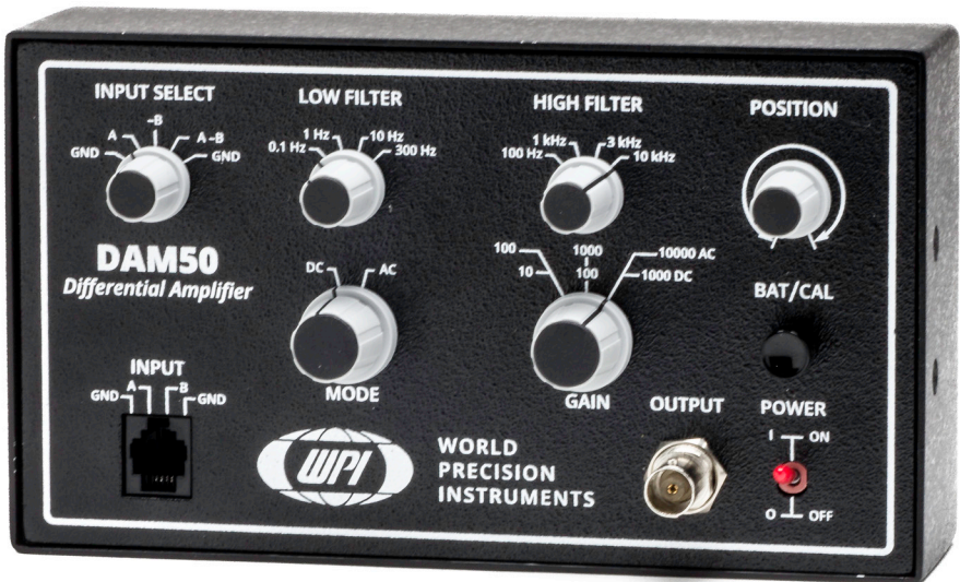
Fig. 1—The DAM50 is a differential amplifier.
