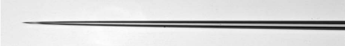
Thick Walled Glass (1.0mm x 0.50mm, BF100-50-10), 0.6-0.9 \mu m tip, 6-8mm taper (400x)
