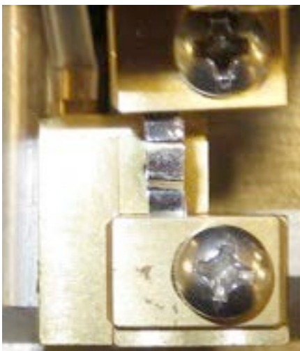
When the filament is installed too far to the right . . . . . the right taper will be longer. MOVE the filament to the LEFT
