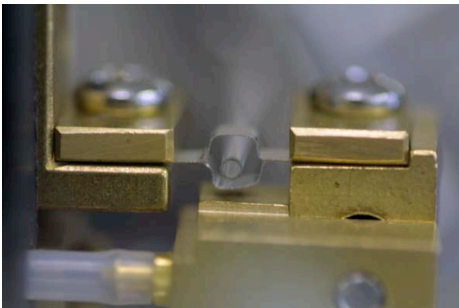
BAD... Air Jet too close
