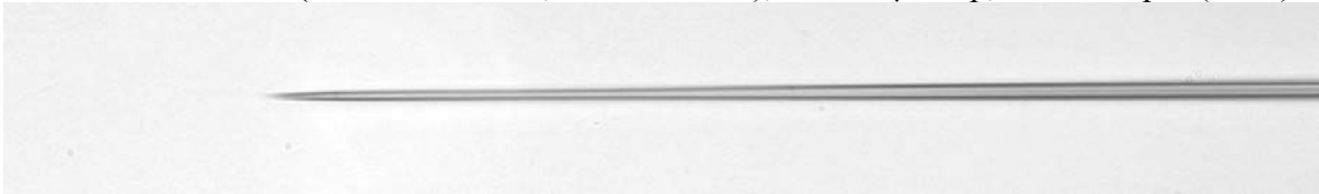
Thin Walled Glass (1.0mm x .78mm, BF100-78-10), 0.7-0.9 \mu m tip, 5-7mm taper (400x)
