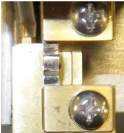
When the filament is installed too far to the left . . . . . the left taper will be longer. MOVE the filament to the RIGHT.
