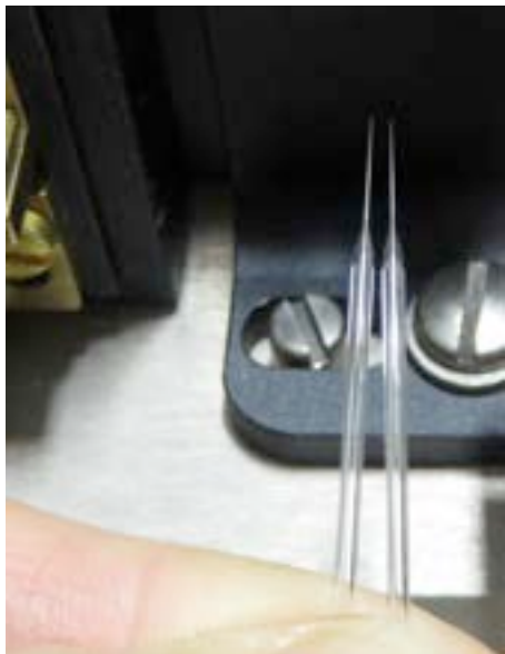
When the filament is perfectly centered over the AIR JET HOLE and centered over the raised brass of the air jet . . . . . ⇒ Both right and left pipettes will be the SAME LENGTH. This is GOOD!
