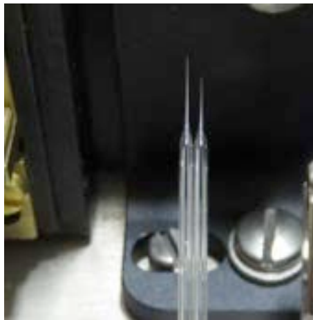
When the filament is installed too far to the left . . . . . the left taper will be longer. MOVE the filament to the RIGHT.
