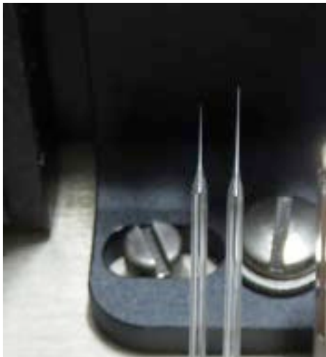
When the filament is installed too far to the right . . . . . the right taper will be longer. MOVE the filament to the LEFT
