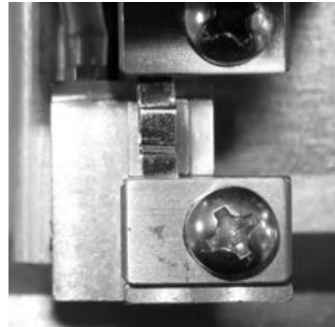
Box Filament Centered Over Air Jet
