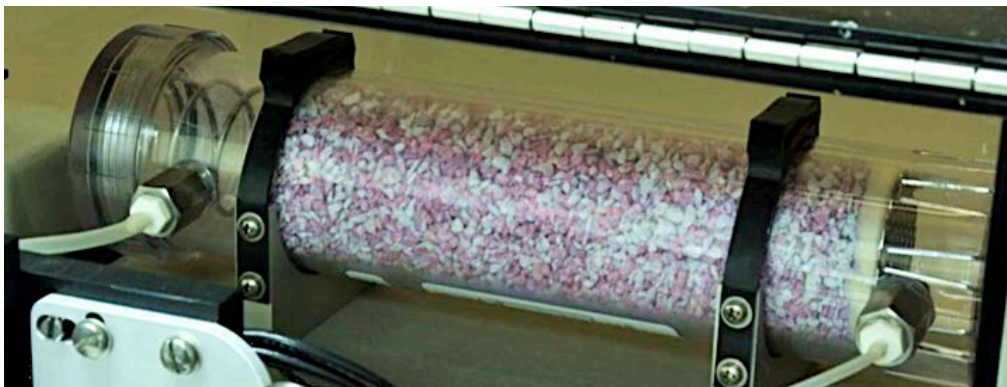
Drierite completely expended... all moist. Time to replace it!
