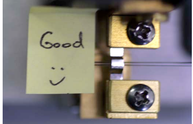
Box filament is centered over the air jet and is 1.0mm in from the left edge of the brass jaws. This is GOOD!
