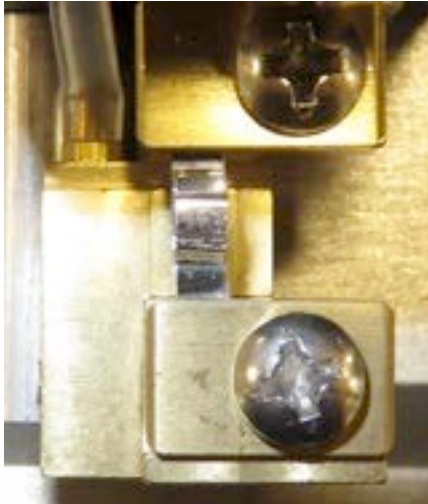
When the filament is installed too far to the right . . . . . the right taper will be longer. MOVE the filament to the LEFT
