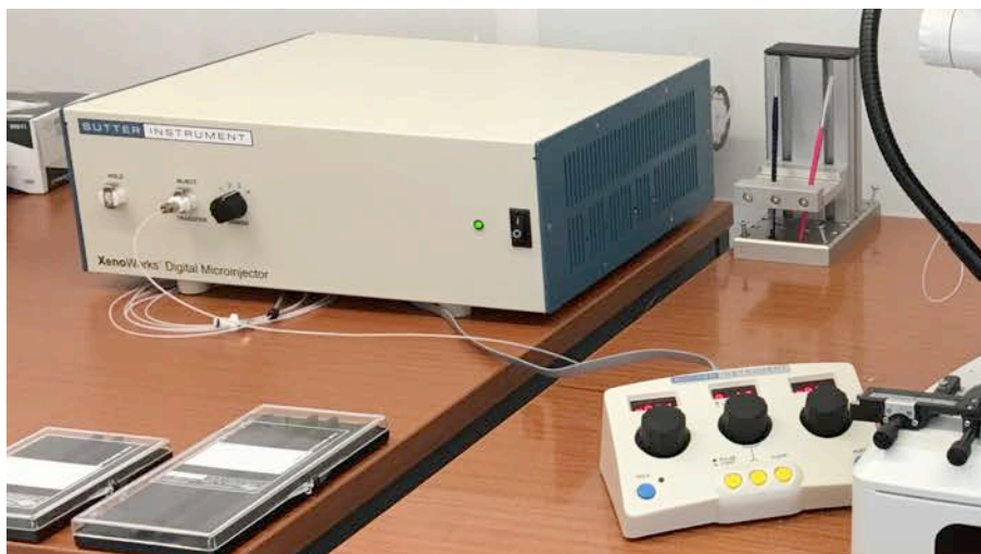
BRE Xenoworks Digital Injector
