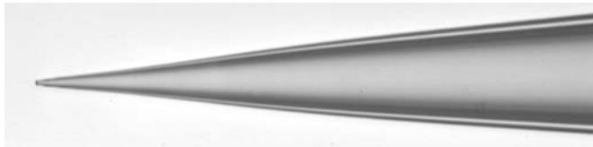
400X mag., 1.5mm x 0.86mm Thick Walled Glass
