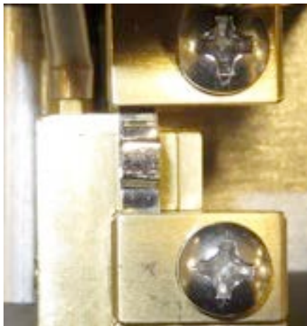
When the filament is installed too far to the left . . . . . the left taper will be longer. MOVE the filament to the RIGHT.
