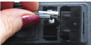
Fig. 7—Open the fuse housing and rotate it right to remove the fuse.
