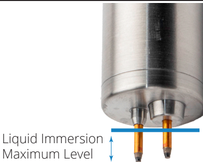
Fig. 5—Don't allow any liquid to pass the line indicated in this image.
