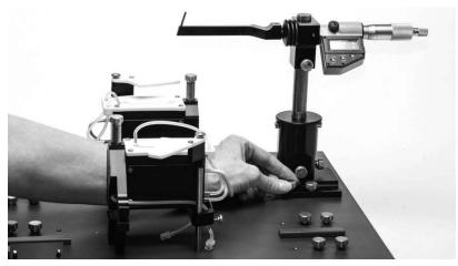
*Fig. 16—Mount the micrometer (motor) stands on the right side using four thumbscrews for each stand.*
