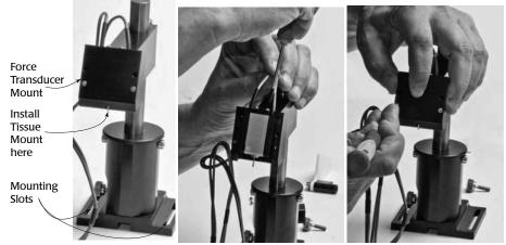
Fig. 22—(Left) Force Transducer Stand
