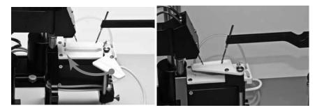
*Fig.* 12—(*Left*) *Rotate the pseudo cuvette into position. Do NOT let the pseudo cuvette damage the tips of the mounting hooks.*
