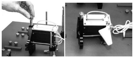
*Fig.* 10—(*Left*) *Reinstall the thumbscrew into the top of the cuvette mounting post. Fig.* 11—(*Right*) *Slide the pseudo cuvette over the pseudo cuvette mounting post.*
