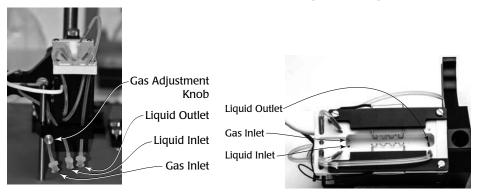
*Fig.* 29—(*Left*) *The side view of the cuvette shows the three tubes for connecting the gas supply and liquid pumps.*
