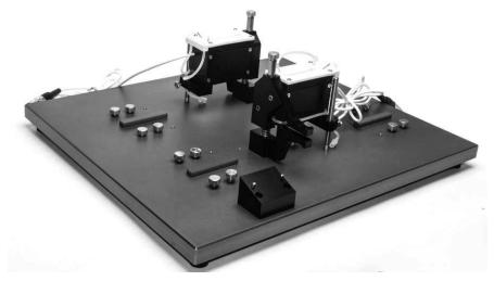
*Fig.* 14—The cuvettes are installed so that the cuvette latches face the outsides of the base plate where they are accessible when you are ready to mount tissues.
