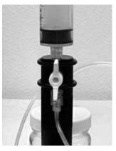
Fig. 36—Syringe valve is in the on position.
