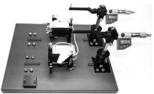
*Fig.* 18—The two micrometers are installed so that the digital displays may be read at the same time.
