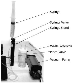
Fig. 31—Vacuum system, labeled parts
