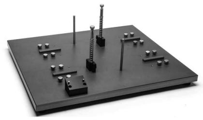
*Fig.* 6—*After installing the cuvette mounting posts, carefully set the base plate down on a flat surface.*
