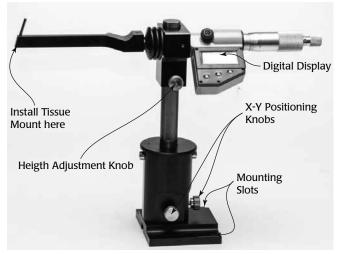
Fig. 15— Micrometer assembly
