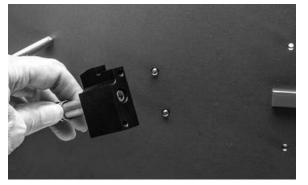
*Fig.* 5—Align the holes on the cuvette mounting post with the holes on the base plate. Make sure that the cuvette latch does not point towards the center of the base plate.
