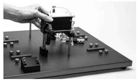
*Fig.* 8—*Slide the cuvette over the mounting posts.*
