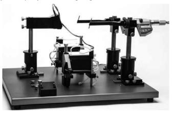
*Fig. 27—Position the force transducer stand on the left side of the base plate.*
