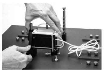
Fig. 9—Pinch the cuvette latch together with one hand and gently press down with the other hand to secure the cuvette in its low position.
