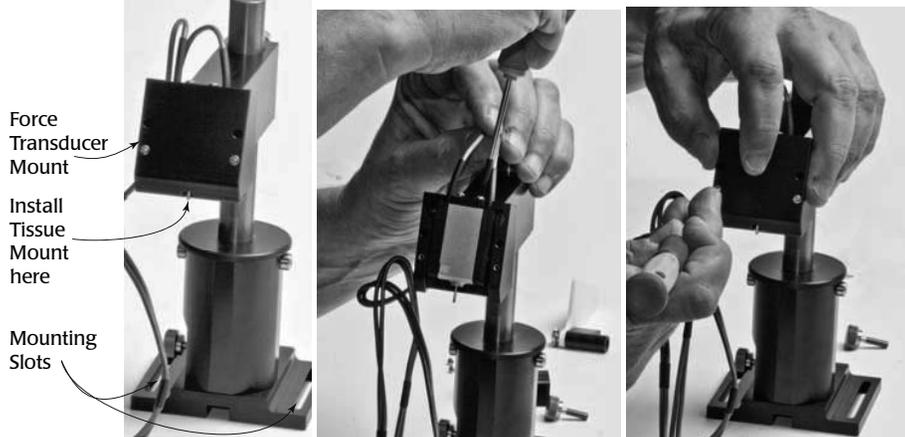
Fig. 22—(Left) Force Transducer Stand
