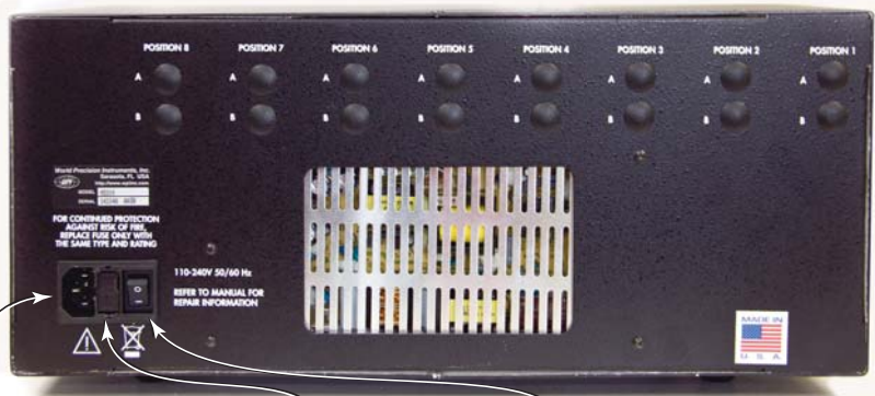
Fig. 4—The back panel of the Signal Conditioning Amplifier System has a master power switch that is usually left on.
