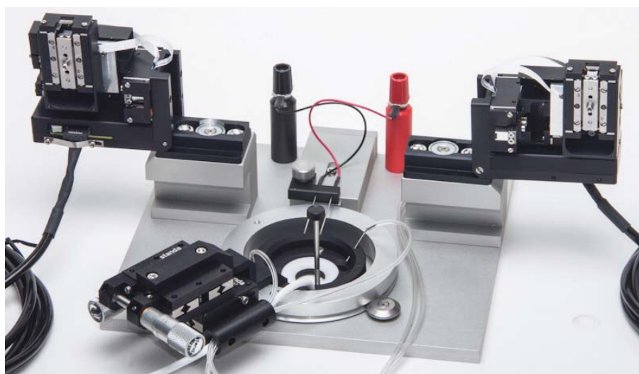
Fig. 23—Both manipulators are mounted and tilted back as far as they can go.
