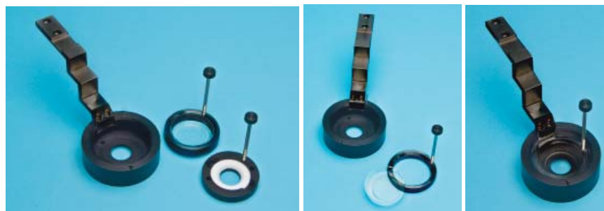
Fig. 12--(Left) The two inserts fit into the rotating stage holder. (Center) The 35mm glass bottom dish fits into the first insert. (Right) The insert and dish are placed in the rotating cuvette.
