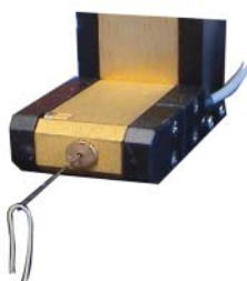
Fig. 33—Suspend a 5\text{mg} weight from the end of the force transducer.
