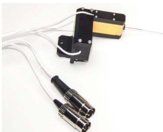
Fig. 6—(Left) The force transducer (sensor assembly) is packaged in a sturdy box to protect the sensitive assembly, and it should always be stored in the case to protect the delicate tip. Fig. 7—(Right) The force transducer has a colored band on one cable to indicate which connector plugs into the Transducer Tweezer port on the Position Control module.
