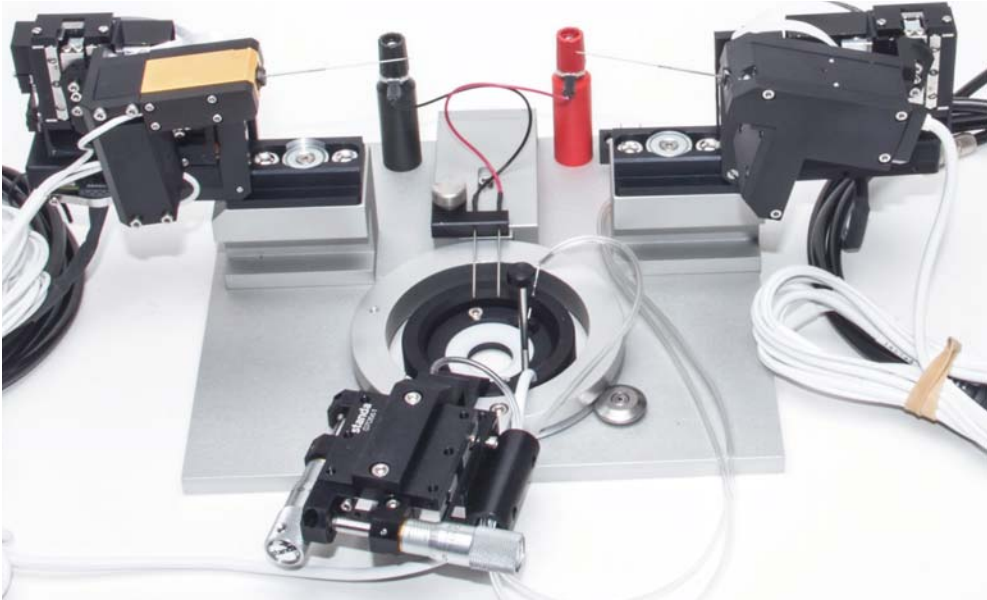
Fig. 27–The force transducer is mounted on the left side and the nanomotor on the right side.
