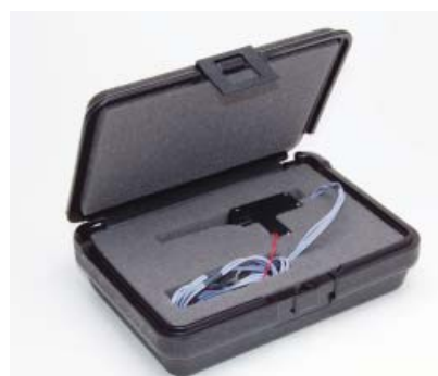
Fig. 6—(Left) The force transducer (sensor assembly) is packaged in a sturdy box to protect the sensitive assembly, and it should always be stored in the case to protect the delicate tip. Fig. 7—(Right) The force transducer has a colored band on one cable to indicate which connector plugs into the Transducer Tweezer port on the Position Control module.
