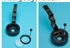
(Left) The 35mm glass bottom dish fits into the first insert. (Right) The insert and dish are placed in the rotating cuvette.
