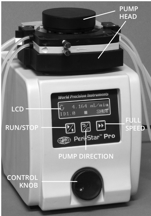
Fig. 2—Pump is labeled.
