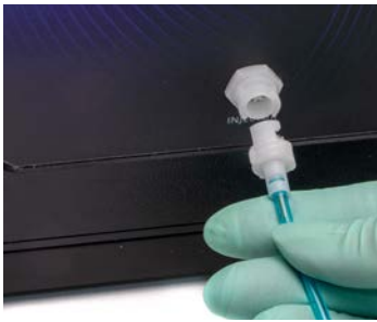
Fig. 12—(Left) Align the connector with the Injection Port, slide the connector in position and rotate the connector a little clockwise to lock it into place.
