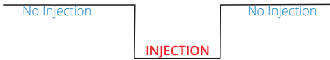
Fig. 15—The injection happens on the high to low transition of the TTL pulse.
