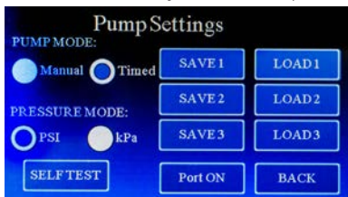
Fig. 24—The Settings menu lets you save enable or disable the Injection Port by pressing the Port ON/Port OFF toggle button.
