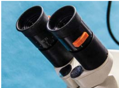
Fig. 30—The orange locking buttons on the side of the eyepieces prevent diopter adjustments from shifting. To change your diopter setting, depress the orange button before rotating the eyepiece.
