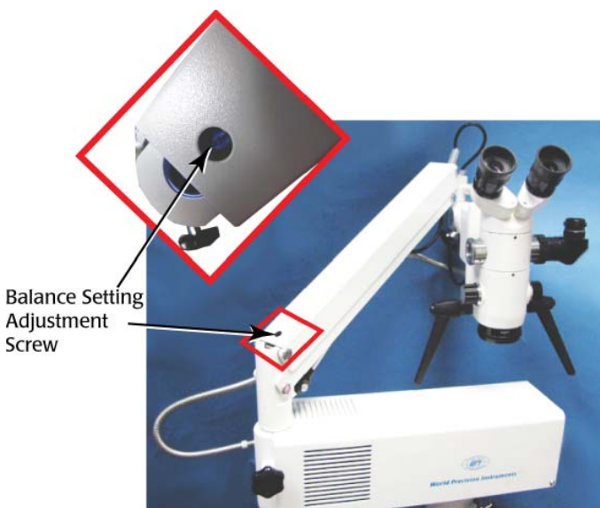
Fig. 33—Location of the balance setting adjustment screw
