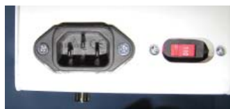
Fig. 2—Voltage switch set to 110V AC
