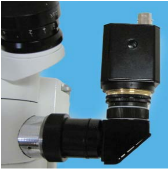
Fig. 22—Camera mounted on the CS-mount coupler
