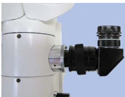
Fig. 19—CS-mount attached to the beam splitter
