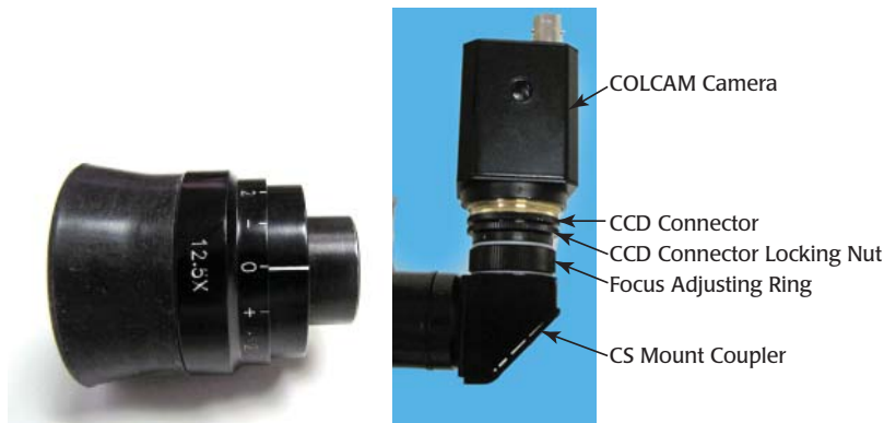
Fig. 24—(Left) Diopters on the eyepiece
