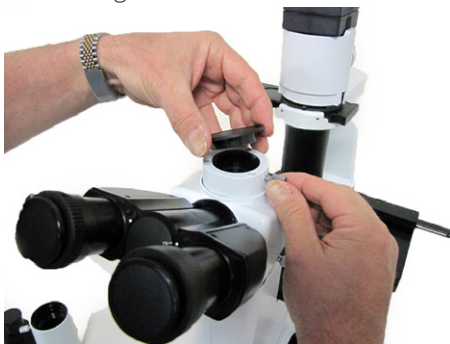
Fig. 32—Remove dust cover
