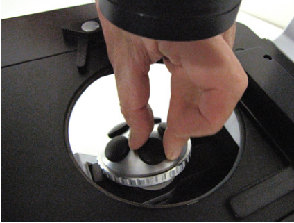
Fig. 38—Removing dust cover to mount objective
