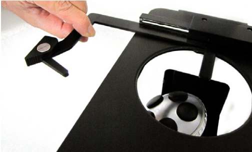
Fig. 13—Extension arm of coaxial stage assembly.
