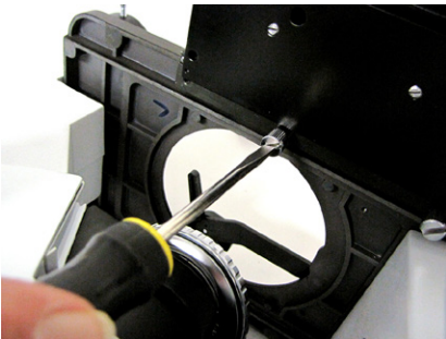
Fig. 10— Fig. 10 —Gently tighten the captive mounting screws.
