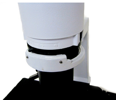
Fig. 18—Condenser in mounting position
