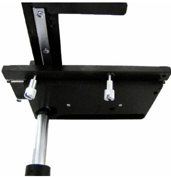
Fig. 7—Captive mounting screws on the coaxial stage assembly
