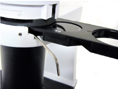
Fig. 65—Insert hex wrench in the right opening
