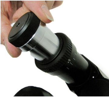
Fig. 61—Phase telescope in eyepiece
