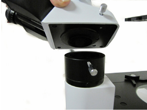
Fig. 30—Position head on the mount
