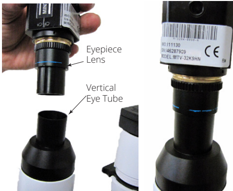
Fig. 70—Line up the camera with tube
