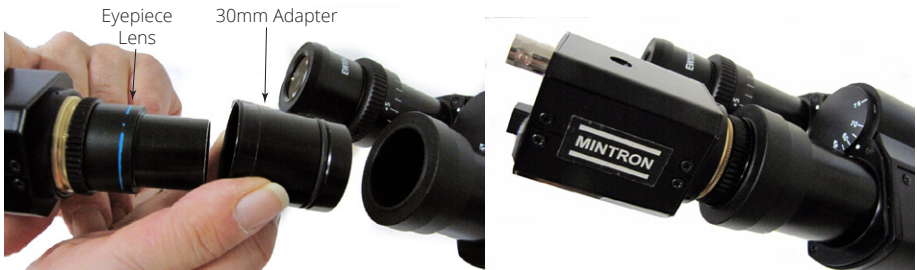
Fig. 72—Camera mounted in eyepiece
