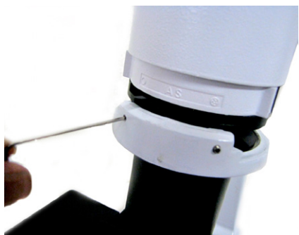
Fig. 20—Tighten hex screws on condenser head
