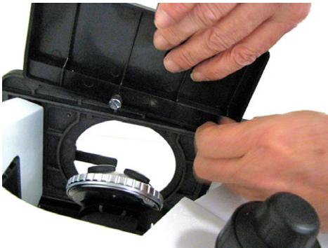
Fig. 14—Left stage plate captive screws
