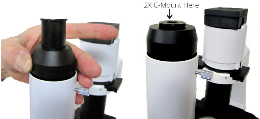
Fig. 34—Eyepiece tube screw mounted
