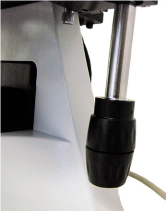
Fig. 78—Coaxial X-Y Control
