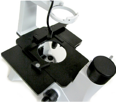
Fig. 16—Coaxial and left stage plate mounted
