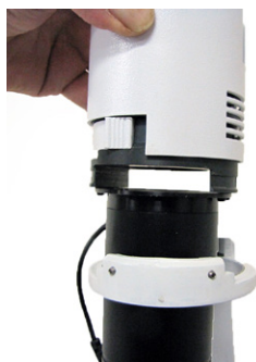
Fig. 18—Condenser in mounting position
