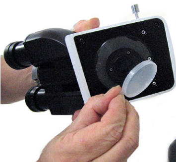
Fig. 28— Fig. 28 —Trinocular head and dust cover
