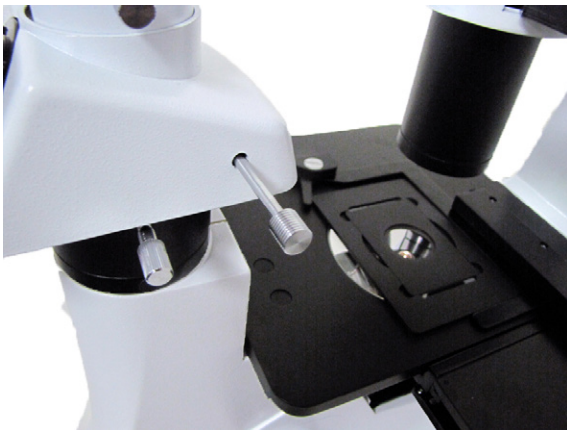
Fig. 77—Switch to enable trinocular extension viewing
