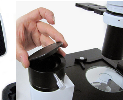
Fig. 28— Fig. 28 —Trinocular head and dust cover
