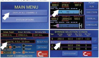
Configure the plunger position – Press the CONFIGURE button to open the Configuration screen. Press the RESET POS button to enter the Syringe Stop Definition screen. Press the WITHDRAW or INFUSE button to set the position of the plunger at the base of the Nanoliter 2020 collet. When you press the WITHDRAW or INFUSE button, you should feel (and hear) the pump
