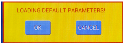
Fig. 51—Warning message appears indicating that you are about to reload the factory default settings.
