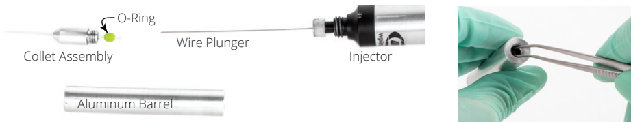
Fig. 13—(Left) The injector is disassembled to replace the gaskets.
