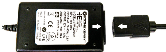
Fig. 17—Connect the power cord to the power supply.
