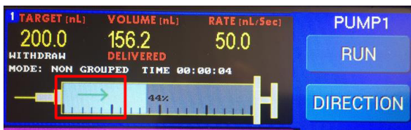
Fig. 42—The arrow indicates the pump is withdrawing. (Example Parameters: Delivery Rate = 200 nL/sec, Volume Target = 3000 nL, Motor Drive= MAX LOAD)
