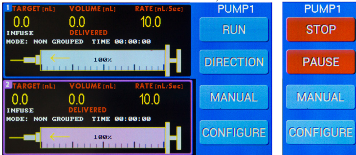
Fig. 7—When the Run button is pressed, it changes to Stop and the Direction button changes to Pause.
