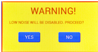
Fig. 50—Warning message appears to let you know that the motors will be re-engaged and the Low Noise Recording period will end.
