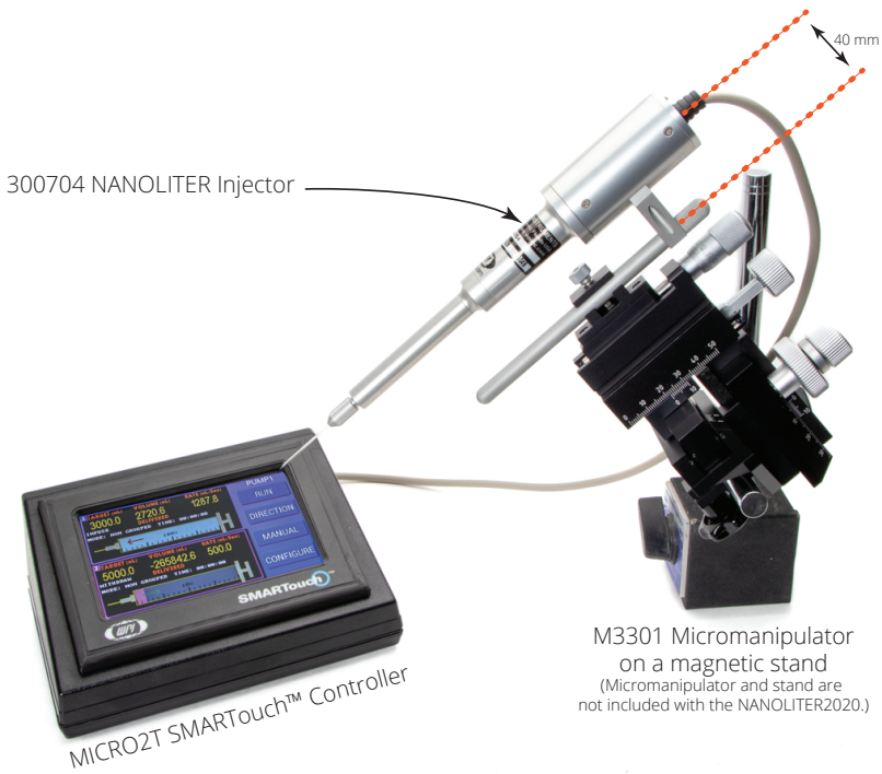
Fig. 2—NANOLITER 2020 System can be used on a micromanipulator which is NOT included with the NANOLITER2020.
