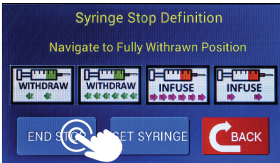
Fig. 33—Press the End Stop button.
