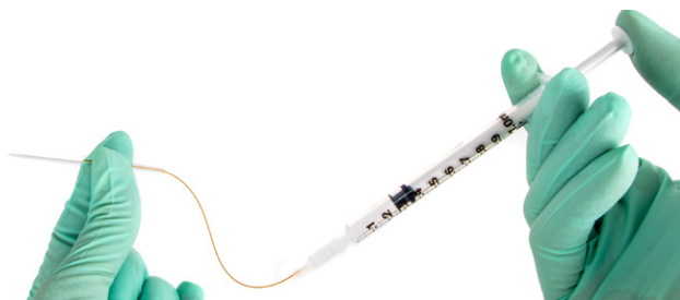
Fig. 35—MicroFil is a thin flexible needle that lets you quickly back fill a micropipette.
