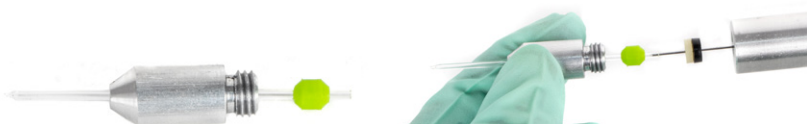
Fig. 36—(Left) Slide the blunt end of the micropipette through the tip of the collet and push it through the appropriate sized O-ring.
