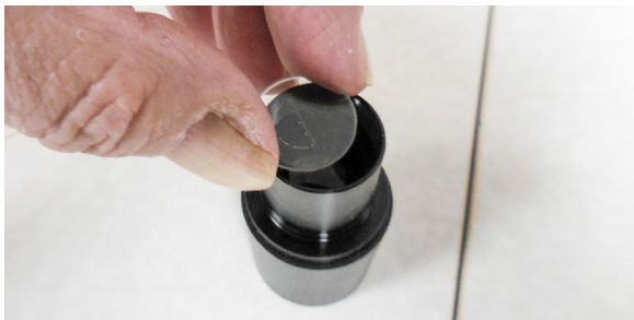
Fig. 23—Insert the reticle with the text on the bottom side of the reticle.
