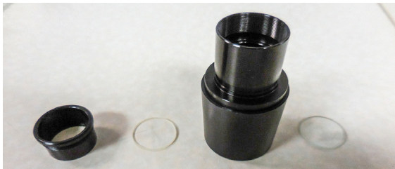
Fig. 22—The reticle ring was removed.
