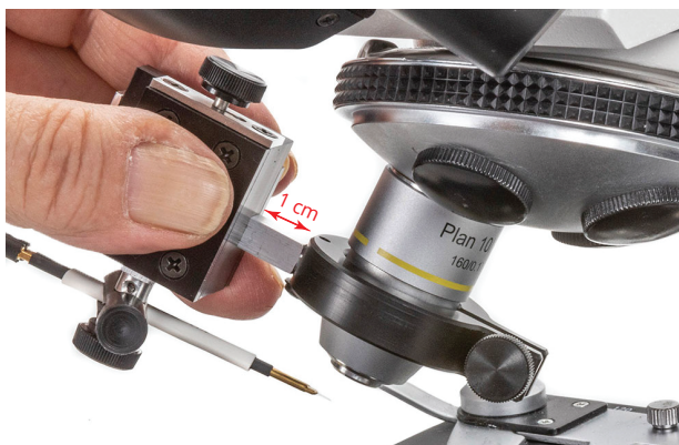
Fig. 6—Mounting the Filament Adjustment Assembly
