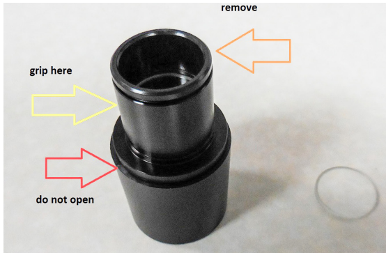
Fig. 21—Loosen the reticle ring.
