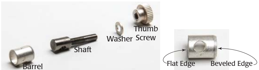
Fig. 2—(Left) The barrel slides over the shaft so that the beveled end is positioned towards the bracket holder and the hole in the barrel is aligned with the hole in the shaft.
