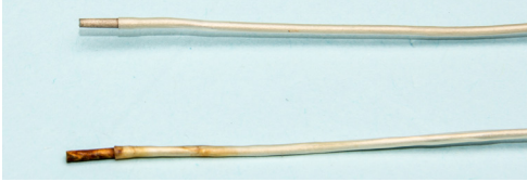
Fig. 5—The good sensor is shown on the top, and the sensor on the bottom has been exposed to the calibration solution for far too long.
