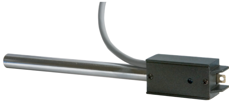
Fig. 1—The FORT transducers have arms around the sensing leaf to protect it.
