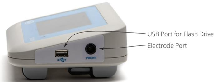
The ports on the side of the unit let you connect a USB flash drive and the EVOM™ electrode.
