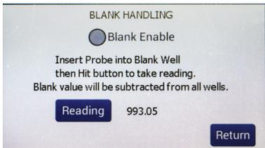
Fig. 48—(Left) Blank Handling window.
