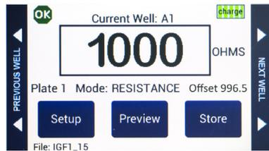
Fig. 49—(Right) The main screen shows the offset underneath the reading.
