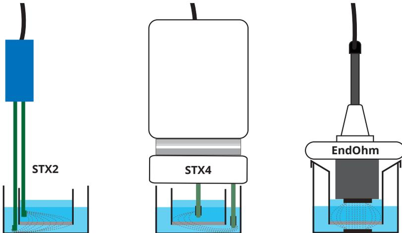
Fig. 73—This comparison shows how the electrode geometry can affect readings.
