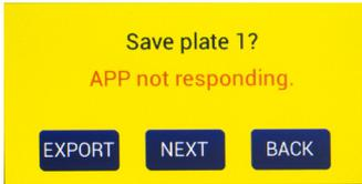
Fig. 32—This message indicates that the data save has timed out. Make sure the unit is connected to the PC and the EVOM™ Companion Application is running on the PC.
