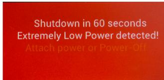
Fig. 65—When the battery power falls to 0%, a warning displays briefly.
