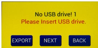
Fig. 59—When the USB flash drive is not plugged in or not recognized, a warning message appears.
