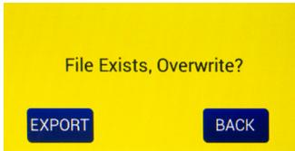
Fig. 26—To overwrite the existing file with the same name, press the Export button. Otherwise, press the Back button, return to the Store Options screen and change the name.
