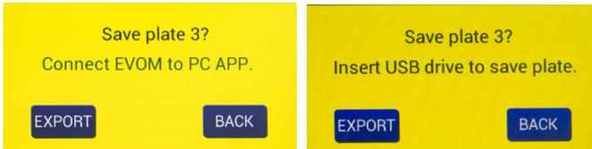
Fig. 60—(Left) After the last cell measurement is taken and you are saving to the EVOM™ Companion Application, this message appears.
