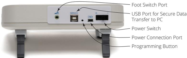
Fig. 4—The ports and controls on the back of the unit let you connect a foot switch, connect a USB cable to a PC for secure data transfer, connect the power adapter, and power on the system.
