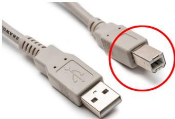
Fig. 72—Plug the USB-B (red) connector into the port on the back of the EVOM™ Manual.
