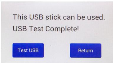
Fig. 42—(Left) The USB flash drive passed the test and is suitable for use with the **EVOM™ Manual**.
