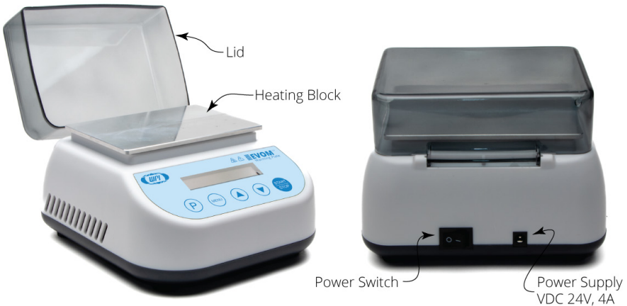
Fig. 2—The front view shows the heating block and the lid used to warm a well plate to 37°C, and the back view shows the power switch and the power supply port.
