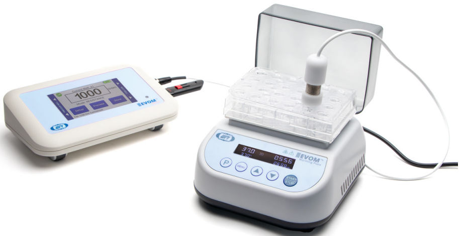
Fig. 6—A 24-well plate is on the plate warmer, and measurements are taken with an STX4 electrode connected to the EVOM™ Manual.
