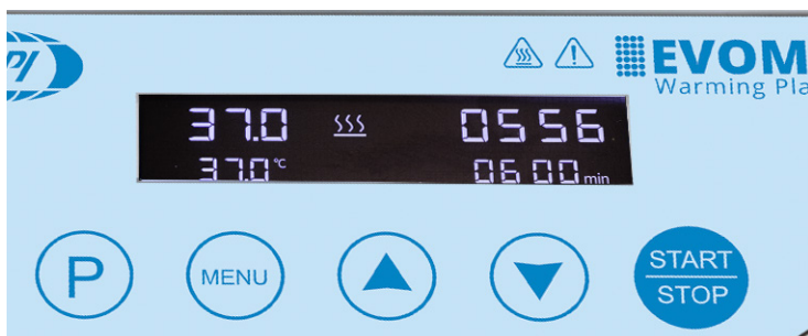
Fig. 5—The Heating Time Remaining starts counting down once EVOM™ Adjustable Warming Plate reaches the desired temperature.
