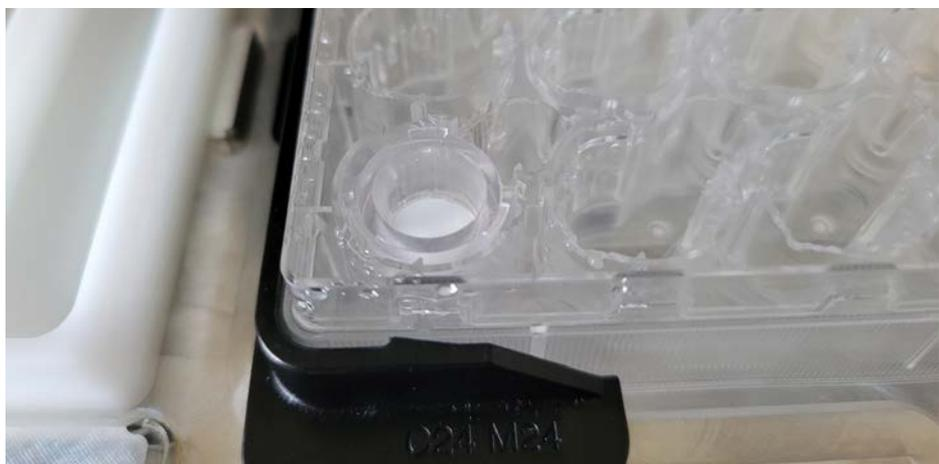
*Fig. 13—MatTek 24 insert improperly placed.*
