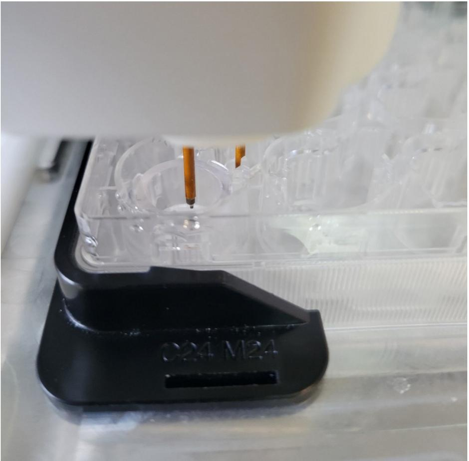
*Fig. 15—Electrodes aligned with MatTek 24 inserts. The electrodes dropped down inside the inserts.*
