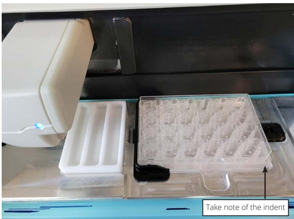
*Fig. 4—Complete Assembly. The Indent should always be in this position to ensure correct plate orientation.*
