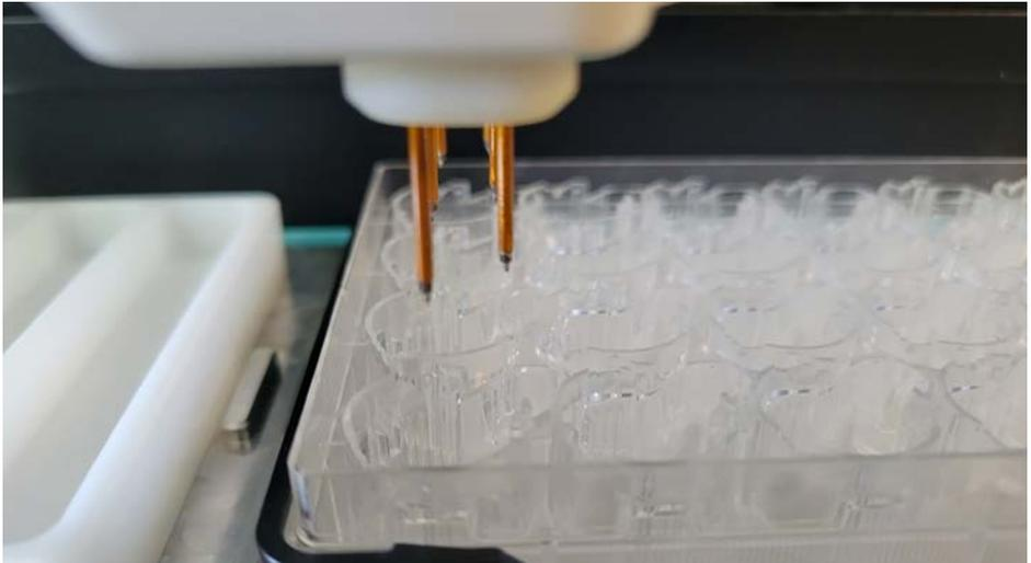
Fig. 6—Electrodes aligned over the Auto Exchange Plate.
