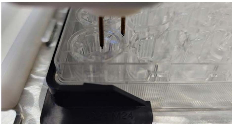
*Fig. 9—Electrodes are aligned with the Auto Exchange Plate with Corning 24 inserts.*
