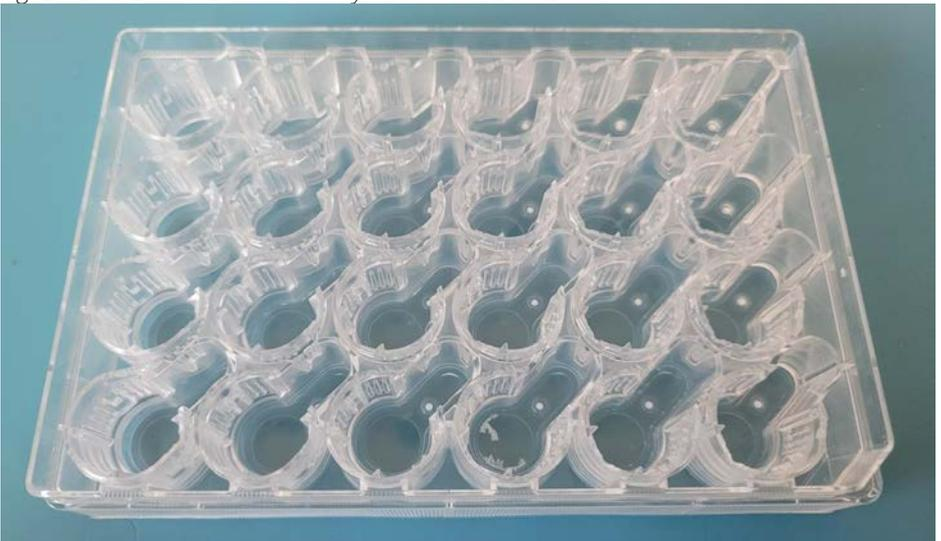
Fig. 3—24-well Auto Exchange Plate. Take note of the indent on the front right corner.
