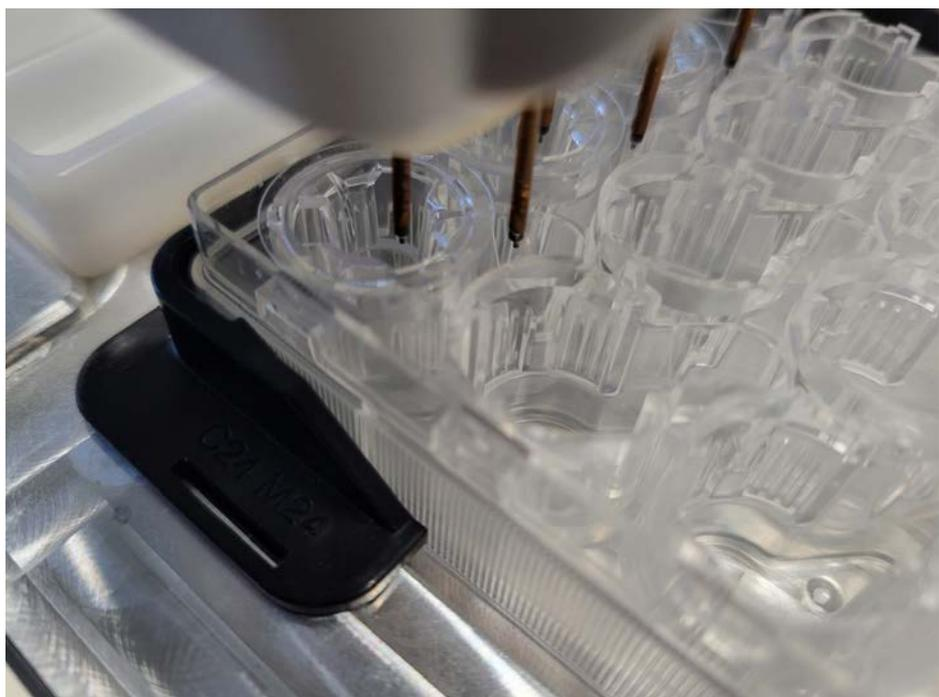
*Fig. 10—Different angle of view of electrodes aligned with the Auto Exchange Plate with Corning 24 inserts.*
