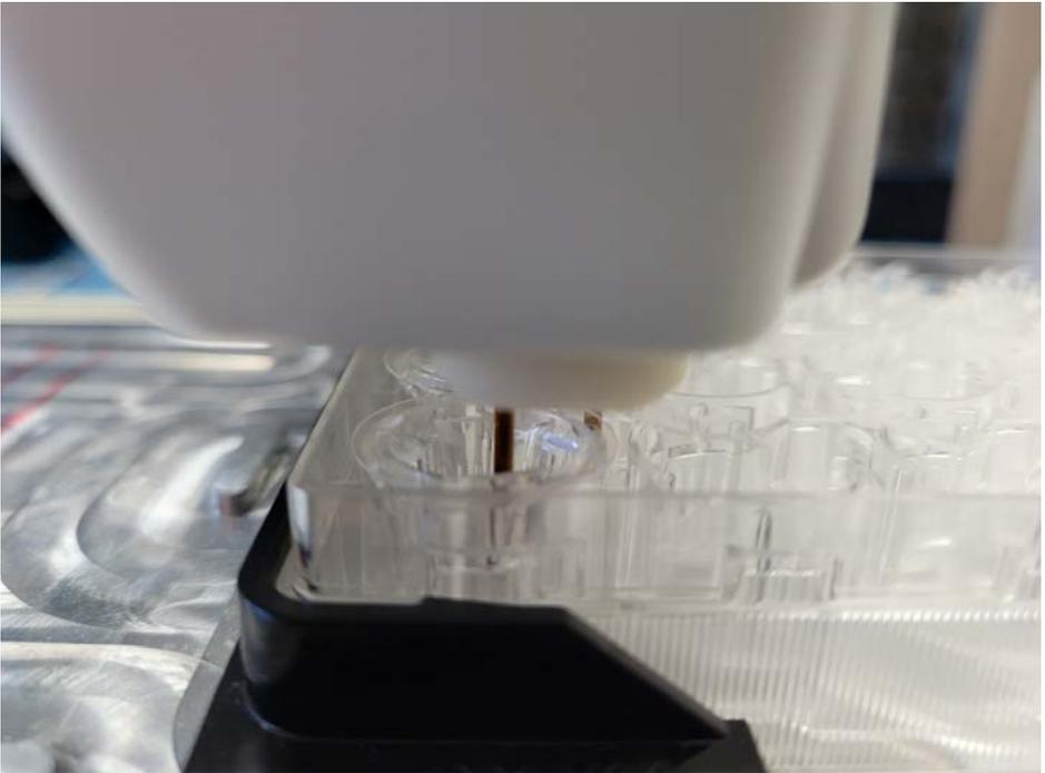
*Fig. 11—Electrodes aligned with Corning 24 inserts. The electrodes have dropped down inside the inserts.*
