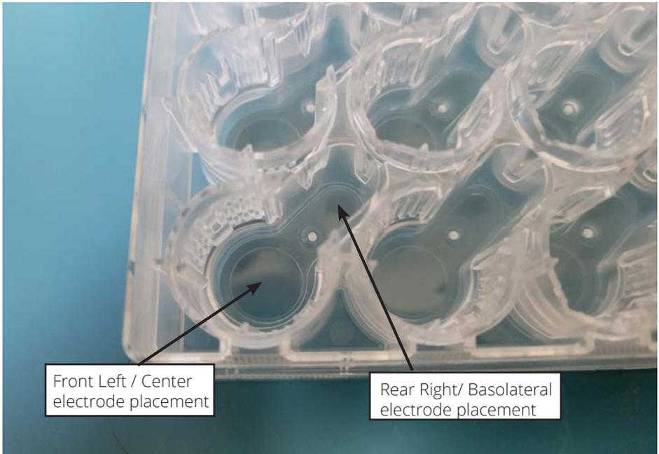
Fig. 5—Close-up of 24-well Auto Exchange Plate.
