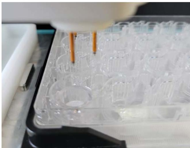
*Fig. 14—Electrode aligned with the MatTek 24 insert.*
