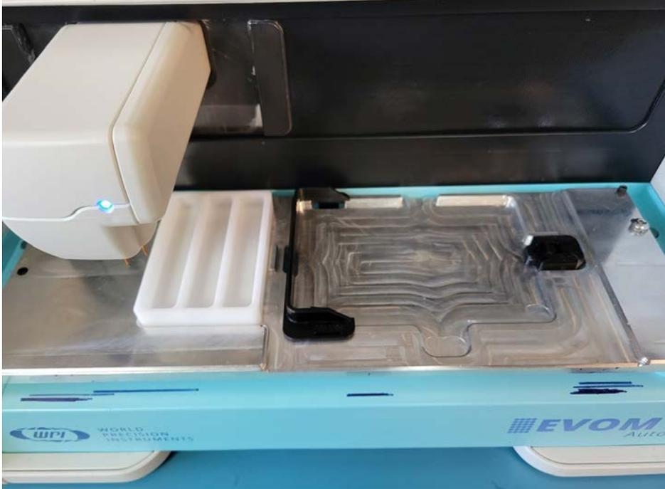
Fig. 2—24M EVOM™ Electrode Array Head and C24/M24 Plate Positioner inserted.
