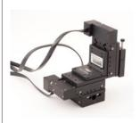
The MP225 features a linear bearings and a modularized, compact design easily adaptable to your setup. 25mm of travel on all three axes with max speed of 3mm/sec.
