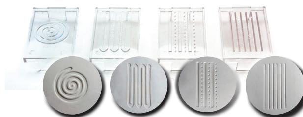
**Z-MOLDS** Microinjection and Transplantation Molds (4 per kit) are designed for zebrafish research. The molds are turned up-side down and placed in liquid agarose gel and are easily removed once it has solidified. Pipette the embryos into the grooves. The embryos self-align.
