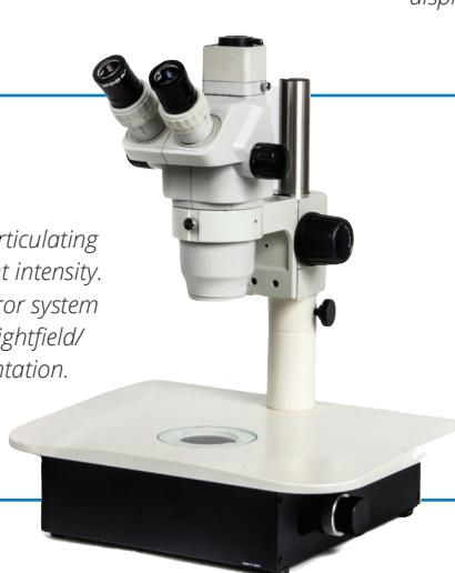
**PZMIII-MI** LED Lighted Microscope Base with articulating mirror and variable light intensity. Dual reflection lens/mirror system provides transmitted brightfield/psuedo-darkfield illumination.
