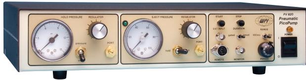
Designed to simplify intracellular injection and a variety of other microinjection tasks, WPI's **PicoPumps** use carefully regulated air pressures for securing cells and injecting them with fluid. Injected volumes range from picoliters to nanoliters.
