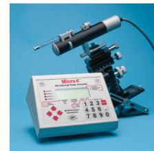
The versatile **UMP3** injector uses microsyringes to deliver picoliter volumes.
