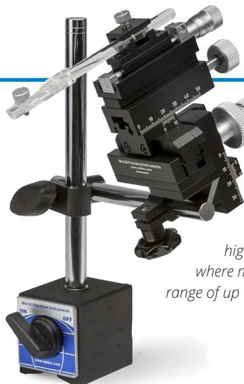
Weighing just 550 grams, the **M3301** is a well-built micromanipulator that outsells all others worldwide for high precision experiments where magnification is in the range of up to 250x.
